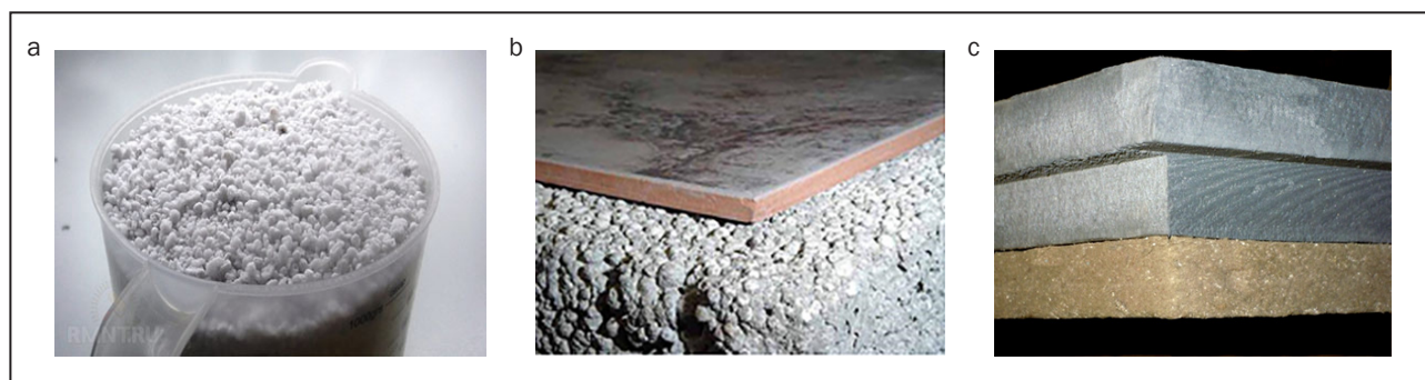
Expanded perlite (a); perlite concrete (b); foam perlite (c)
