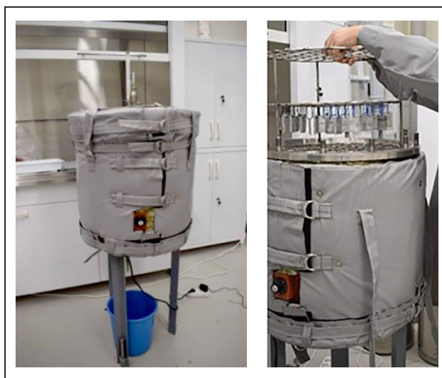
Fig. 2. Appearance of a corrosion test stand
