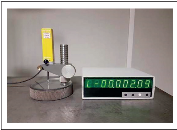
Fig. 2. Holographic DG-30 length meter with access to an autonomous display unit
