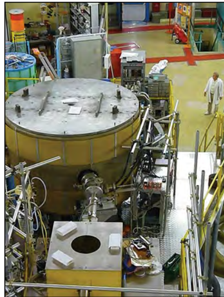
PNPI spectrometer used for the neutron electric dipole moment search at the ultracold neutron beam of the Institute Laue–Langevin
